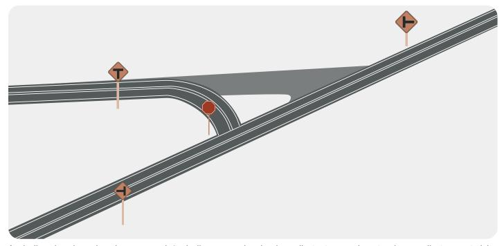
A misaligned or skewed roadway approach (typically a more minor local or collector type roadway to a larger collector or arterial type roadway) creates sight issues for motorists and increases crash risk to all roadway users, including pedestrians and bicyclists. Realignment countermeasures including repaving, striping, signage, and roadway configurations provide better sight distance and visibility at the intersection for all users.
